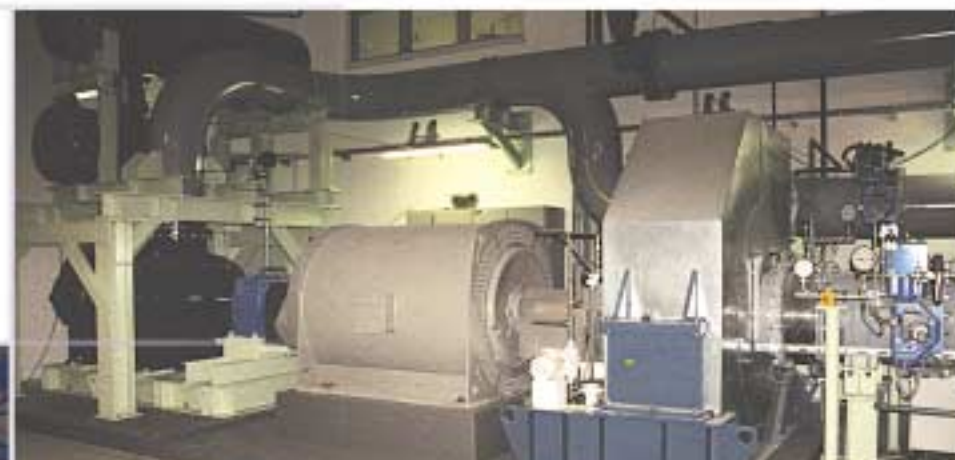
Two stage vacuum pump-set, air cooled 60000 m 3 /h, final vacuum 250 mbar
