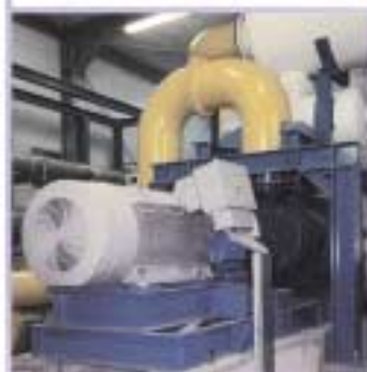
Single stage air preinlet cooled rotary lube blower, 24000 m 3 /h, final vacuum 400mbar
