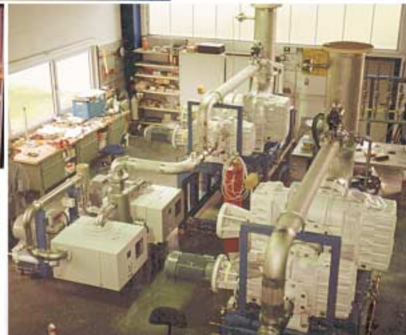
Multistage fine vacuum pump-sets 9000 m 3 /h, final vacuum 1-10 -3 mbar
