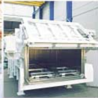
Pressure-shock-resistant sterilisation chamber
