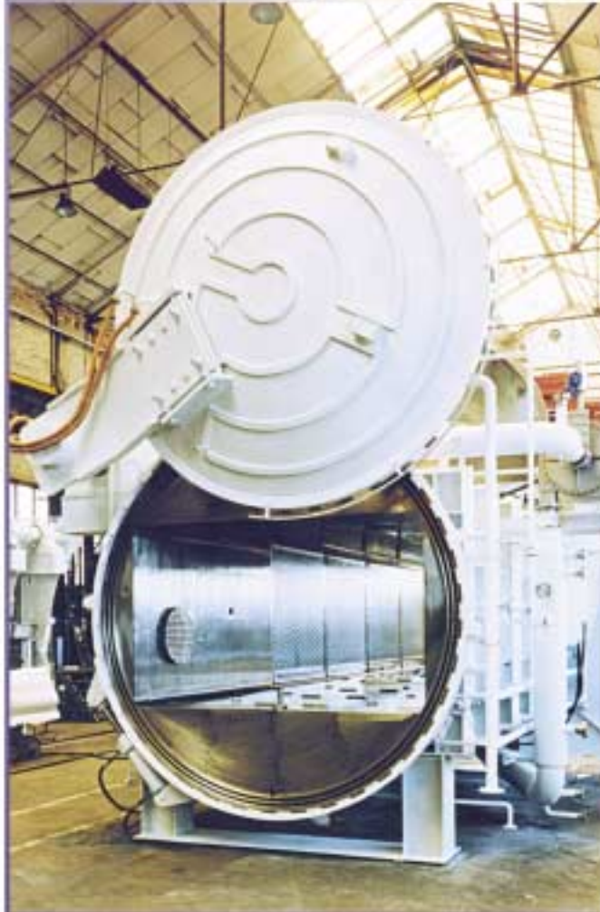
Pressure-shock-resistant sterilisation chamber
